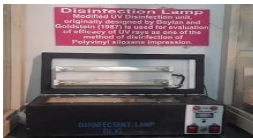
Fig.3 U V light chamber
